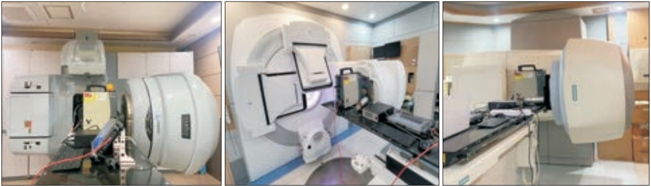
Fig. 2. Setup of the in-situ high-purity Germanium detector in front of the linear accelerator crosshair and relevant measurements.
