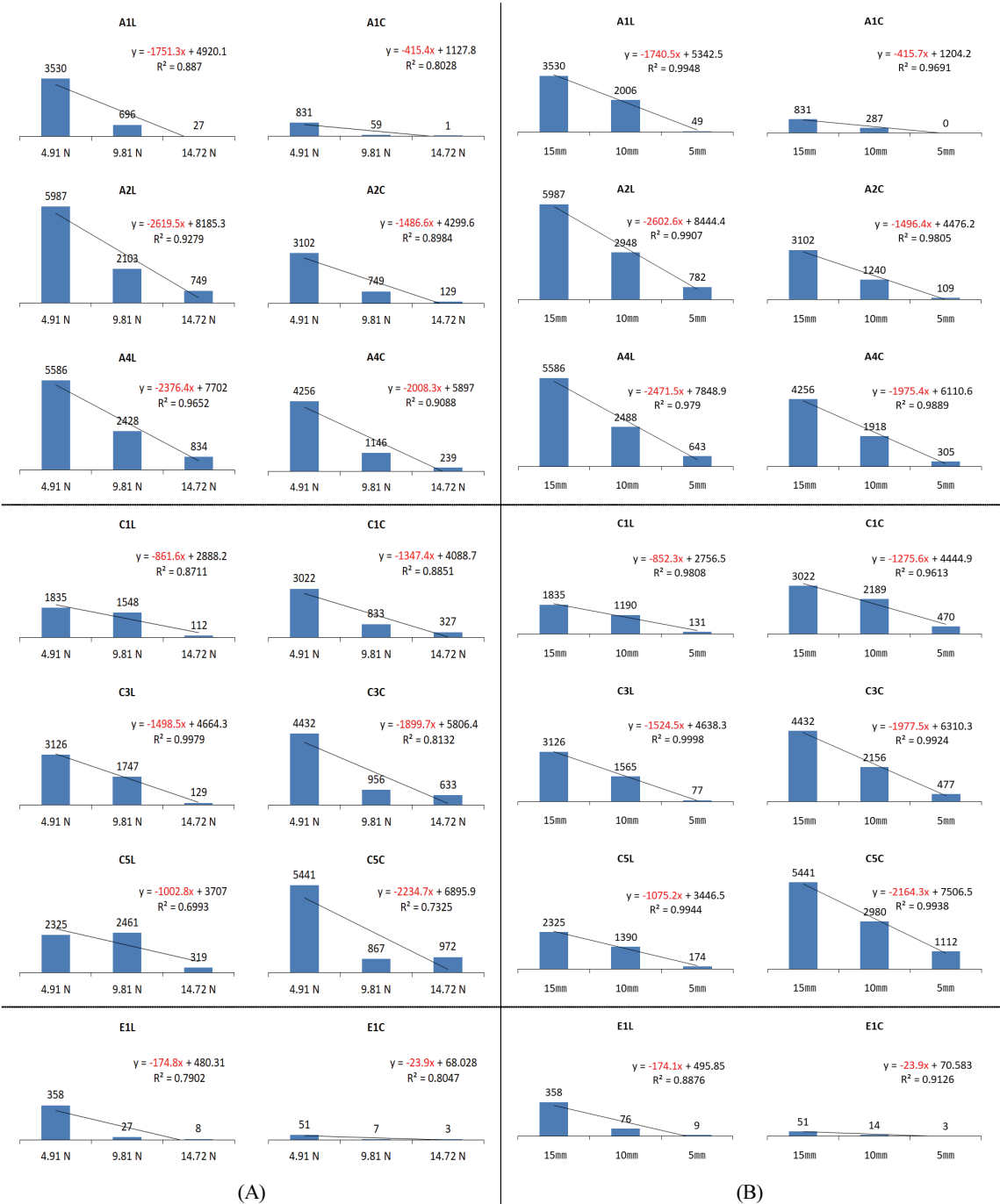
Figure 6. Trend line for folding endurance results of total Hanji. (A) Load conditions. (B) Specimen width conditions.
