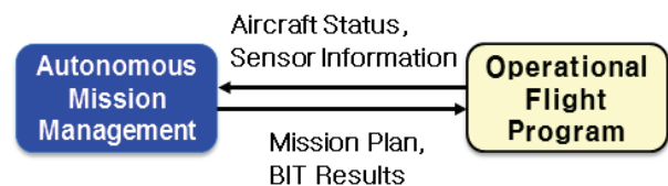
Fig. 1. Inter-communication between Autonomous Mission Management and Operational Flight Program (OFF)
