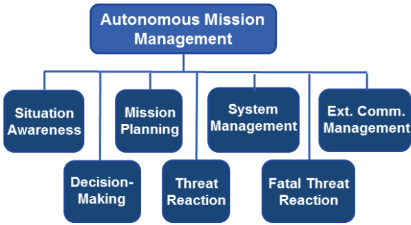
Fig. 2. Autonomous Mission Management software architecture
