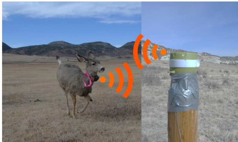
Fig. 1. Base station data collection between a deer collar node and a listener node
