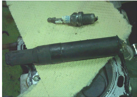
Fig. 3. Damaged example of the spark plug and ignition coil.
