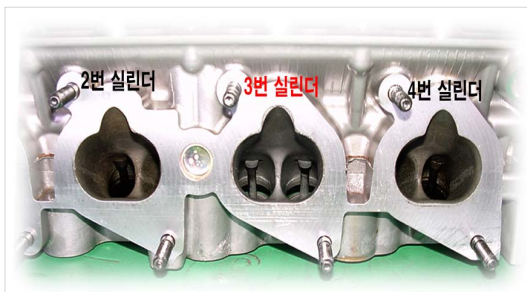
Fig. 9. Combustion chamber shape of the cylinder head
