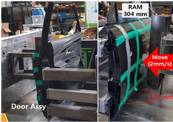
Fig. 13 Experimental set-up for Static side GFRP impact beam protection test(FMVSS-214)
