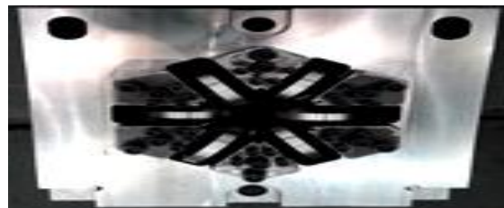
(b) Hexagonal rolling die fixed roll Fig. 2 Drawing system for manufacturing SUS hexagonal bar
