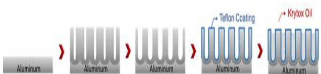
Fig 1. Schematic procedure for sample preparation with anodic oxidation, pore widening, Teflon coating and oil-impregnation..
