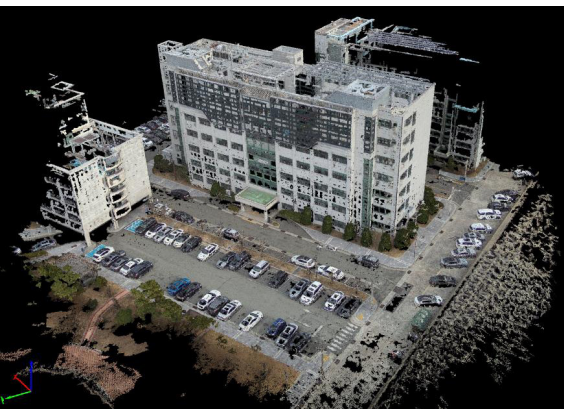
Fig. 7. Dense point cloud from visible images
