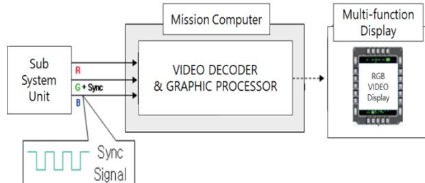
**Fig. 6** RGB and Sync signal from sub-system.
