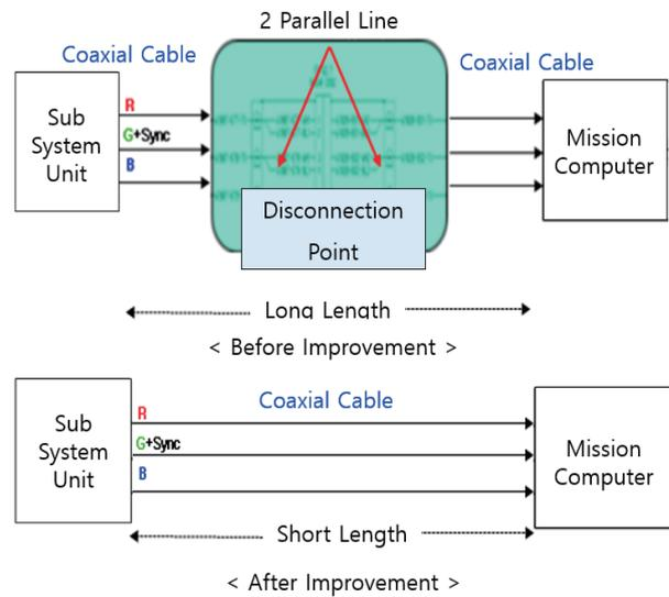
**Fig. 13** Improvement in cable configuration.
