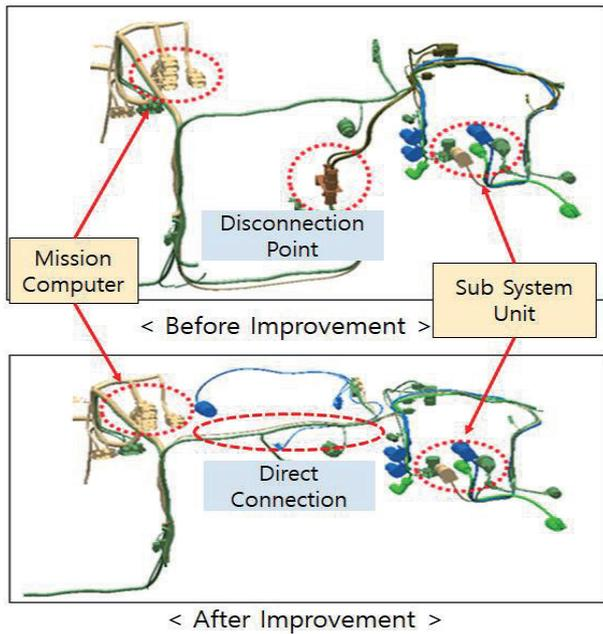
**Fig. 15** Applied wire harness path in the system.
