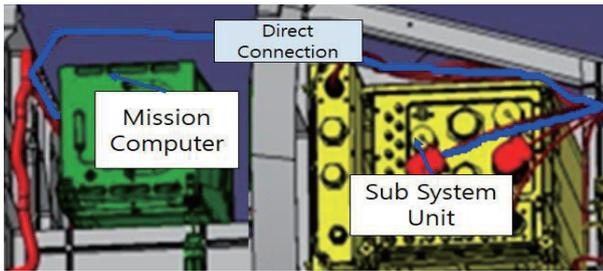
**Fig. 14** Wire harness of RGB signal with direct connection.
