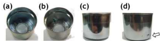
Fig. 1 Magnetic switch case for starter motor A model ((a), (c)) and B model ((b), (d)) appearance photos
