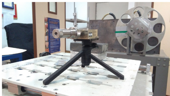
Fig. 3. A CdTe detector for x-ray spectroscopy on the radiometric bench (The detector side is in a tungsten EXCV collimator from Amptek Inc).
