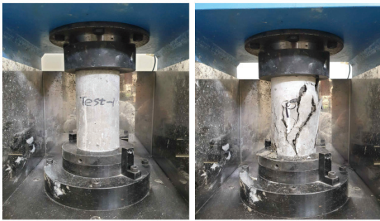
Fig 2. Concrete compressive strength test
