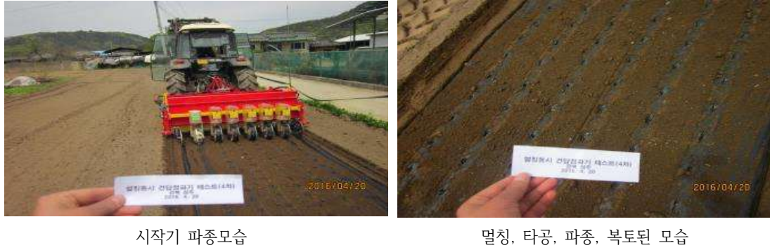
Fig. 4. A view of dry hill seeded rice by mulching dry hill seederII(4th test)
