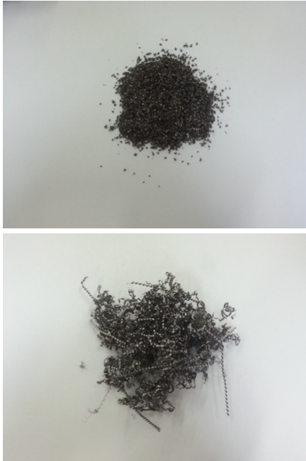
Fig. 2. Shape of chipped titanium scrap obtained after (a) milling and (b) turning.
