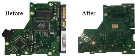
Fig. 7. The photos of PCB before and after SnCl 4 leaching.
