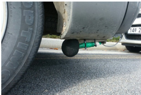
Fig. 2. CPX Noise Measurement; Rear Microphone
