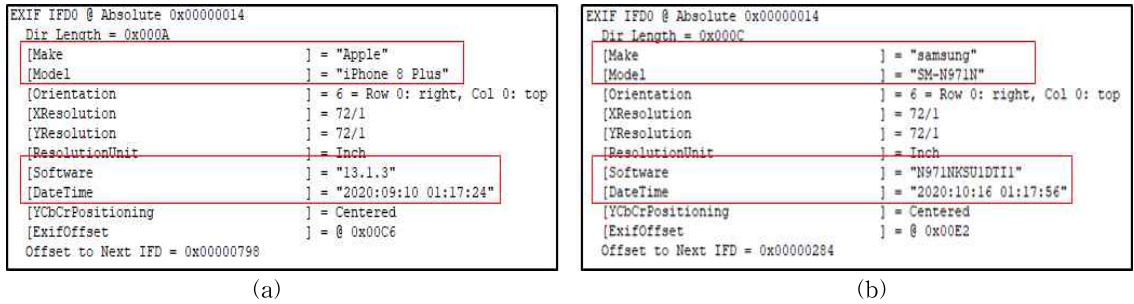
Fig. 4. The example of EXIF information, (a) iPhone 8plus and (b) Samsung note 10 5G.
