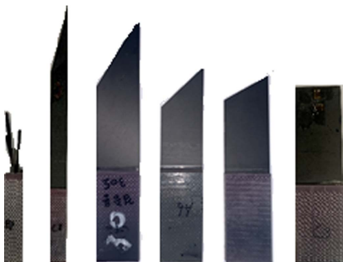
Fig. 4. Failed off-axis composite specimens for fatigue tests
