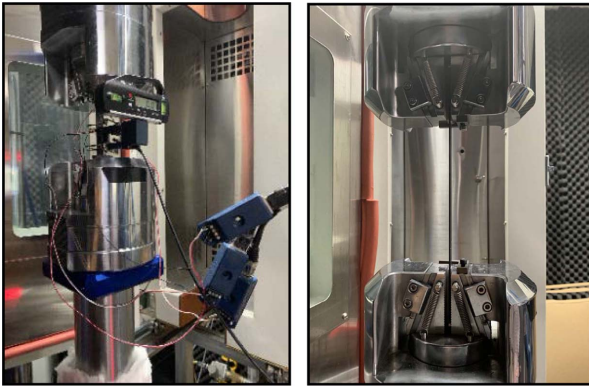
Fig. 3. Experimental setup for tensile and fatigue tests
