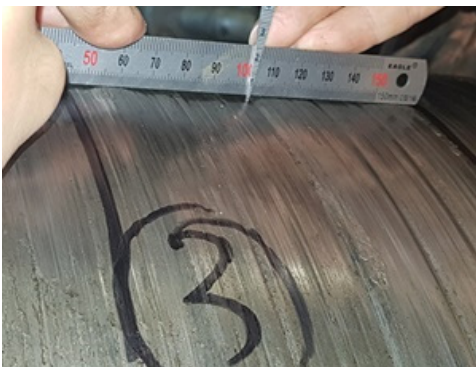
Fig. 4 Propeller shaft damage
