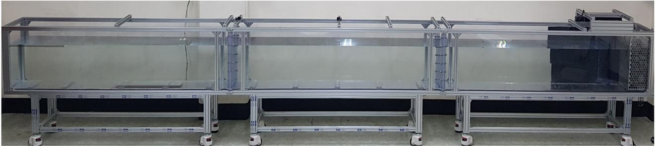
Fig. 2 Overview of Two-dimensional mini wave tank
