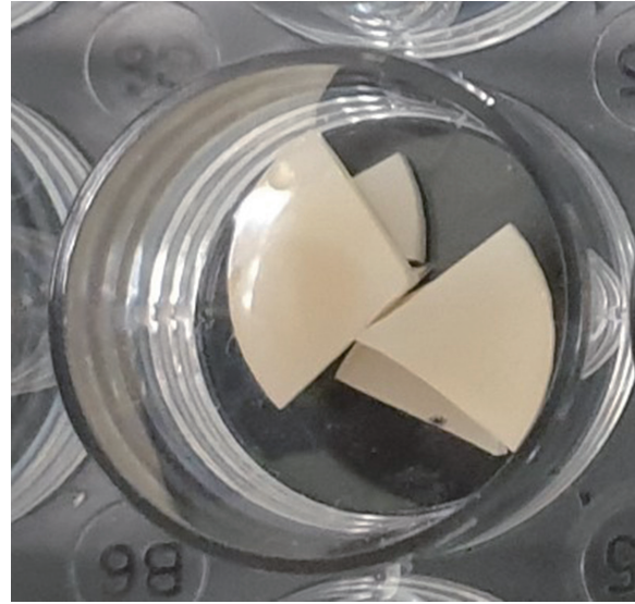
Fig. 5. Specimens were fractured into several pieces in the shape of a fan around the point where the pressure was applied.
