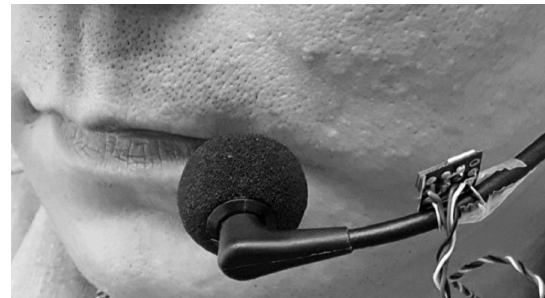
Fig. 1. Photograph of the ultrasonic Doppler sensor, mounted on the right cheek of the subject.
