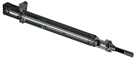
Fig. 14 Final assembly design of cryogenic submerged pump for localization development
