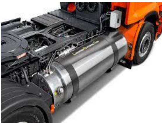
Fig. 1 LNG fuel tank system for commercial vehicle
