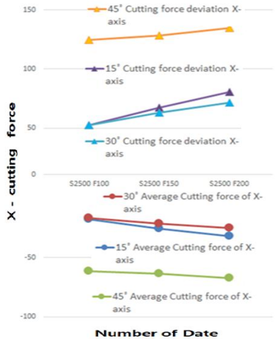
Fig. 7 Measured cutting force of x-axis for upward machining for inclined surface
