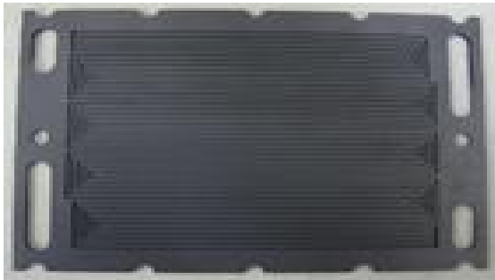
Fig. 4 Bi-polar plate design integrated with gasket
