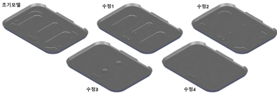
Fig. 7 Design modification of the sunroof considering the shape bead arrangement
