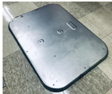
Fig. 9 Stamping product of the modified part design
