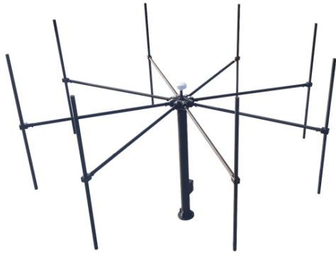
Fig. 2. Configuration of UCA for multistatic PCL
