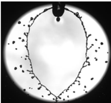
Fig. 3 Typical liquid sheet and droplets
