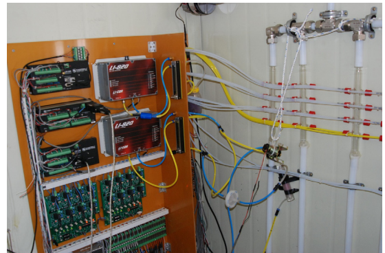
Fig. 3. Photography of the central module of multi-channel automated chamber systems (MCACs) developed for continuous measurements of soil respiration rate in the field.
