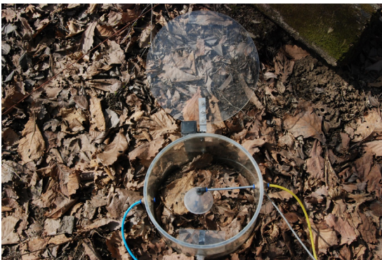
Fig. 2. Photography of the multi-channel automated soil chamber installed at the Nam-san experimental site in a Quercus mongolica forest.
