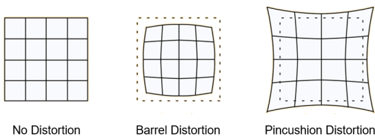
Fig. 1. Lens distortion of the camera.
