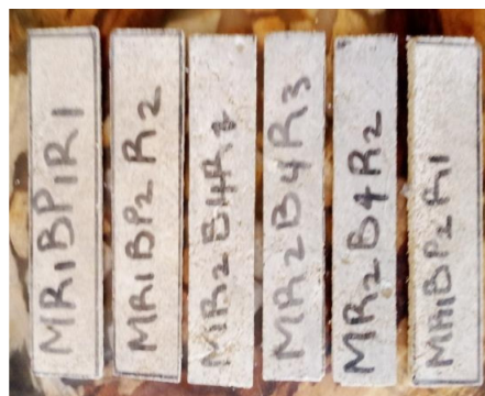
Fig. 4. Board samples for MOE and MOR test.
