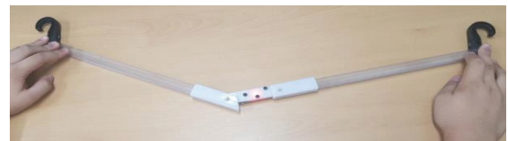
(b) Working mode of greenhouse snow load sensor
