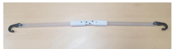
(a) Standby mode of greenhouse snow load sensor
