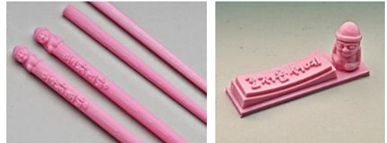
Fig. 21. 3D Printing chopsticks & tray for Dolhareubang (Printed as PLA filament)
