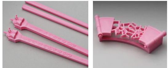
Fig. 17. 3D Printing of chopsticks & tray for King Sejong (Printed as PLA filament)
