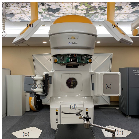
Fig. 5. Novalis Tx (Varian, USA) (a) Exact X-ray detector(Brain Lab, USA) (b) Exact X-ray source(Brain Lab, USA) (c) On-Board Imager(Varian, USA) (d) Reference star to use Exact system(Brain Lab, USA)
