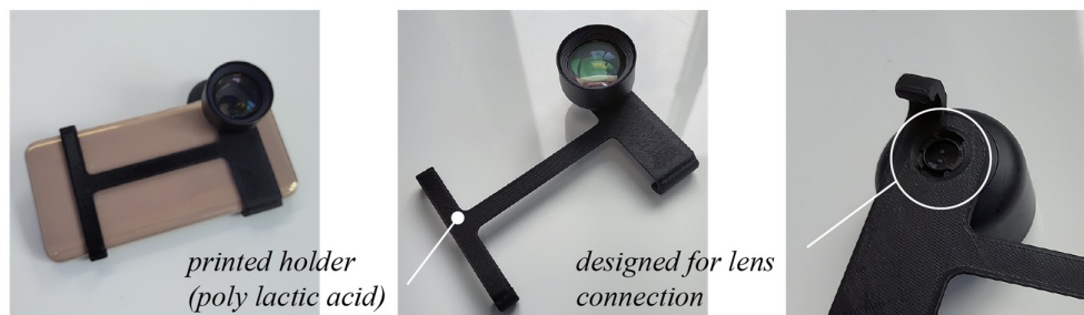
Fig. 3. 3D printed lens holder for smartphone (GW)
