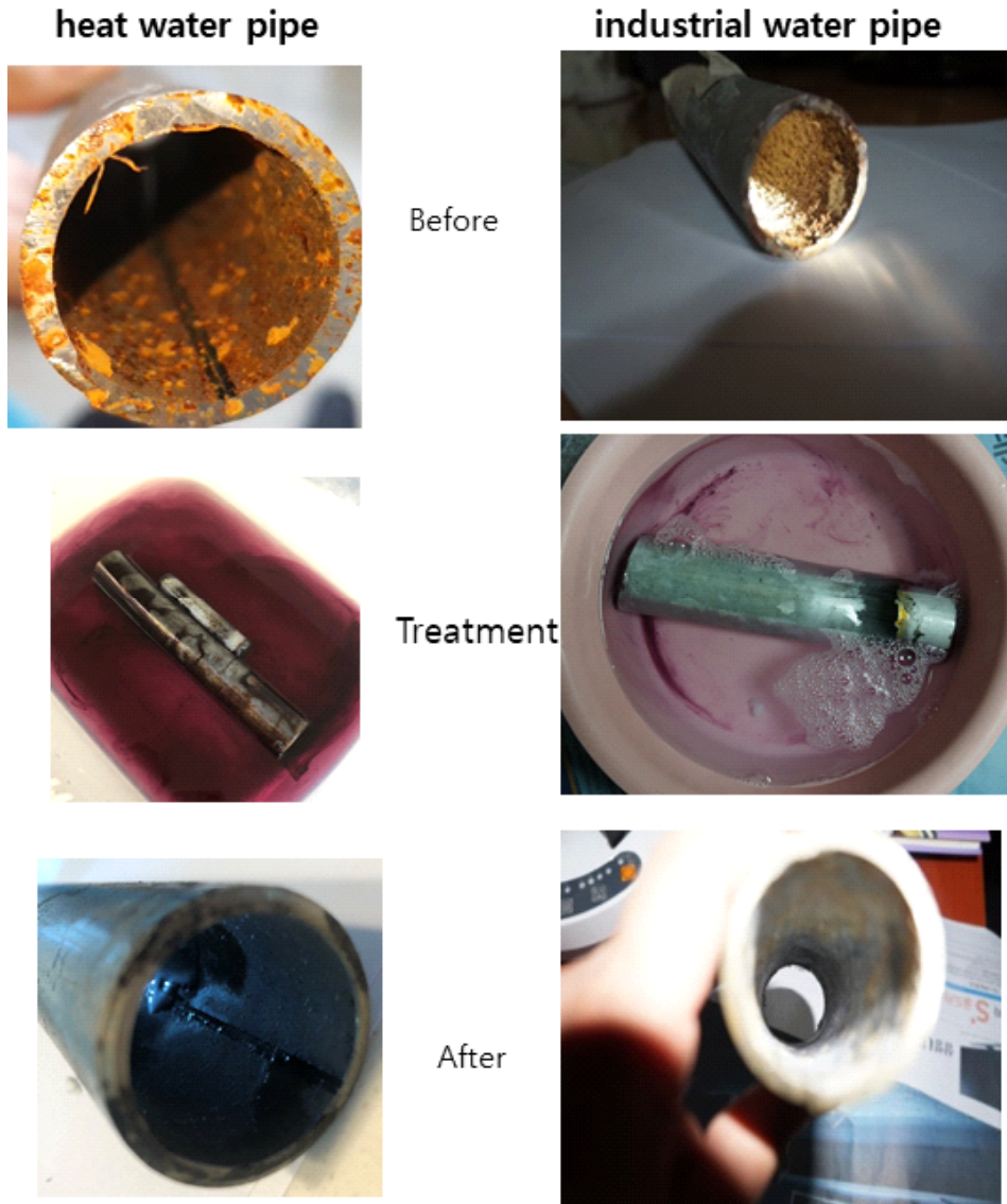
Fig. 5. Photograph of scale removal before and after processing of pipes.
