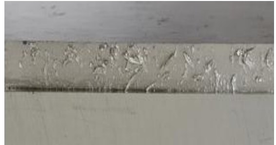
Fig. 11 Surface photo of the cutting surface after upward cutting
