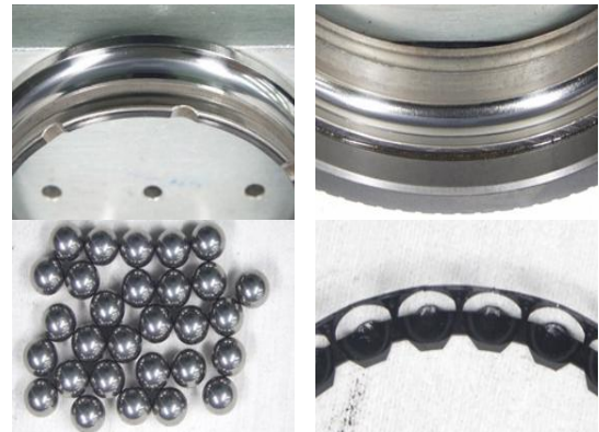
Fig. 8 Bearing inspection after rating life test
