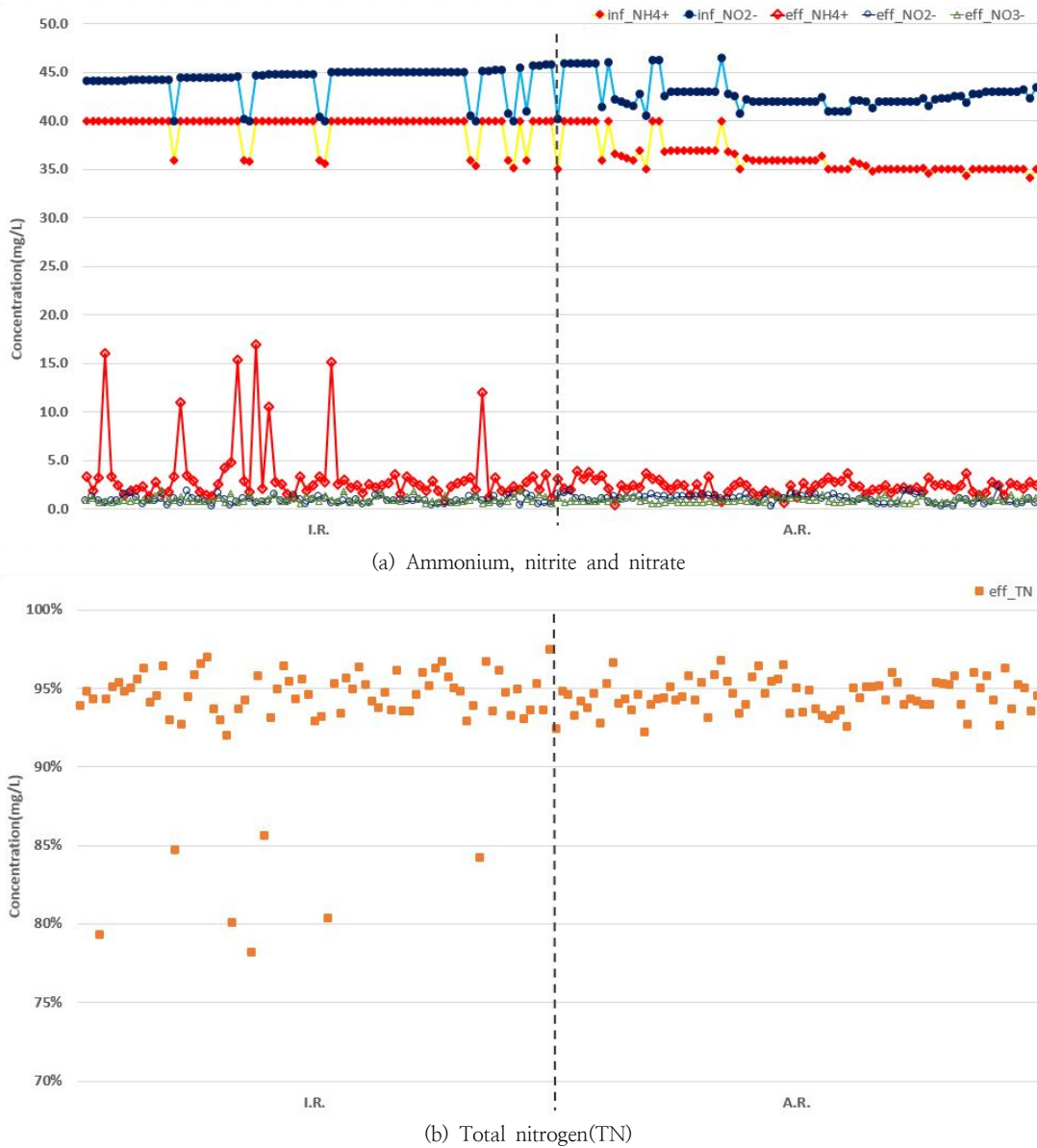
Fig. 2. Operation result of laboratory scale ANAMMOX reactor.
