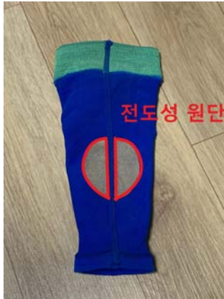
Figure 10. Adhesion of Conductive Fabric on the Inner Side of the Calf Supporter (taken by authors)
