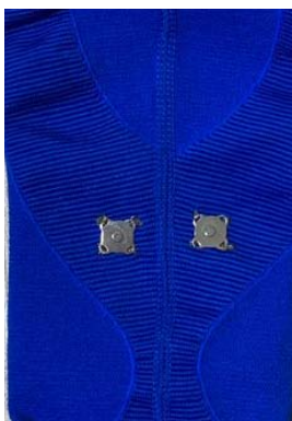
Figure 8. Attaching a Magnetic Snap for the EMS Module (taken by authors)
