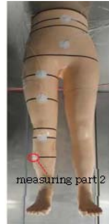
Figure 7. Measuring Part 2, Anterior Tibial Central Measurement Point (KATRI, 2020)
