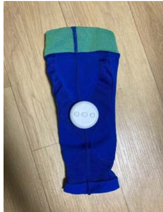
Figure 11. Completed Pressure EMS Supporter Outside (taken by authors)
