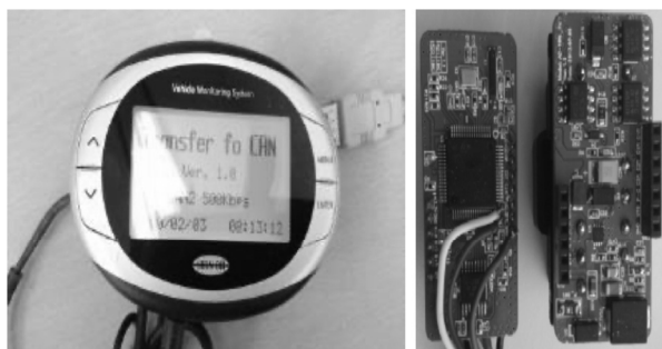
Fig. 3. OBDDI Device Display and PCB Hardware
