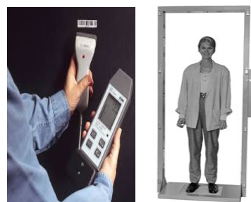
Fig. 1. Two types of survey meter. left: Hand held survey meter Right: transportable portal monitor
