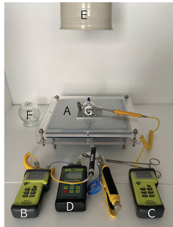
Fig. 2. (A) Skin model. (B) Digital thermometer 1: Temperature inside the cup & skin model. (C) Digital thermometer 2: Temperature at the skin model surface. (D) Digital manometer. (E) Infrared irradiator. (F) Glass cup. (G) Valve cup
