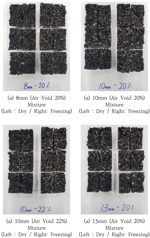
Fig. 3. Specimen Splitted after Indirect Tensile Strength Test
