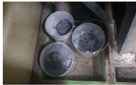
(a) Specimen Freezing at -18^{\circ}\text{C} for 16hours
