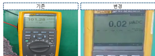
Fig. 20. Measured result of leakage current about Improved point in Monitoring board
