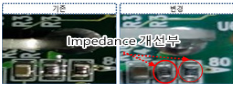
Fig. 21. Improved Battery voltage detector in control board
