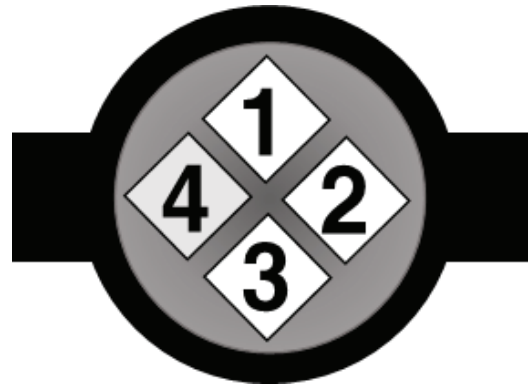
Fig. 1. Schematic of the substrate holder used in the ion beam sputter (number denotes the position of each substrate).
