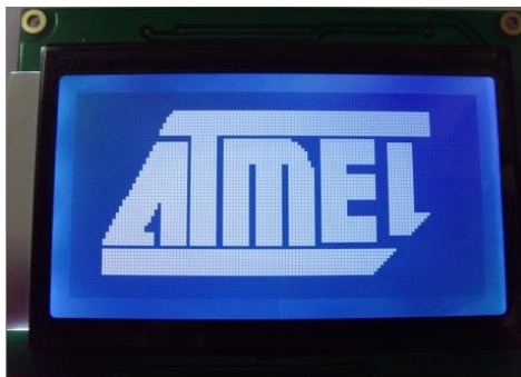
Fig. 5. 12864 Graphical LCD Module, [Source]excerpt from the web page https://avrmall.com
