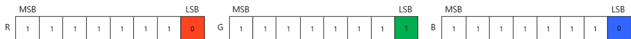
Figure 1. Sample Confidential data embedding in LSBs of R, G, B components of a pixel
