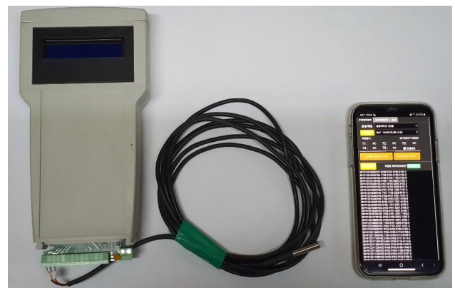
Figure 3. Concrete IoT management system
